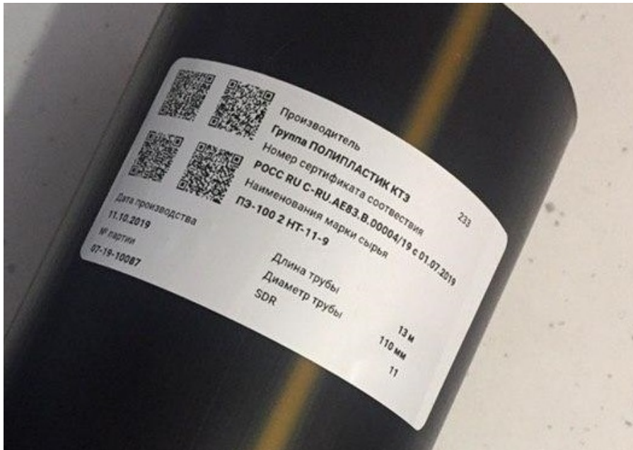
Figure 7 — Plastic pipe with a label (in Russian)
